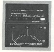
attenuator system is used (OPTI-RANGE). With this feature, you need only set a single range control for an on-scale indication. A second control is provided for situations where the automatic system may not be suitable, as with some measurements of transient signals.
